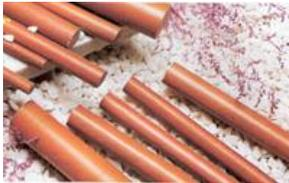
**PHENOLIC CLOTH LAMINATING ROD** Phenolic cloth laminating rod is made of cotton cloth , impregnated with phenolic resin and hot pressed with forming dies . This rod possesses high mechanical property , suitable for use as insulating parts for electric equipment . It can be used in transformer oil
