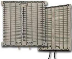
Toaster Elements are made from high grade Mica paper Board, Natural Mica. Nickel Chrome Resistance wire for its longer life. These elements are mainly used in pop-up toasters in house hold appliances.
